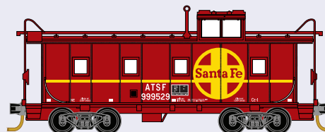
36' RIVETED STEEL CABOOSE, OFFSET CUPOLA - ATSF #999529
